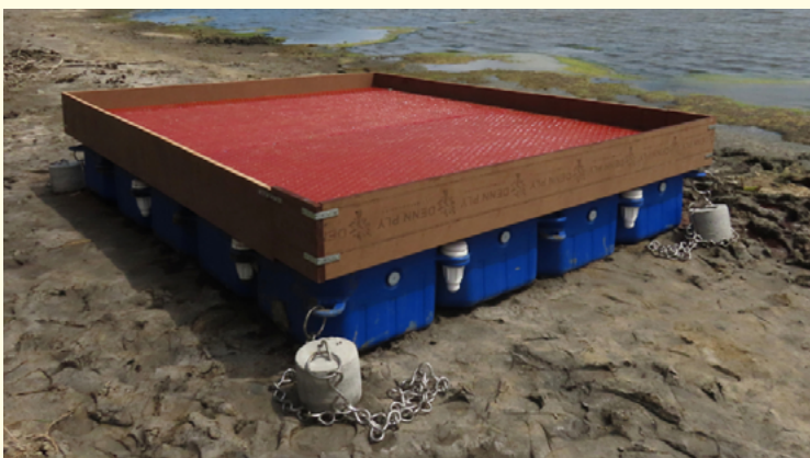
Four concrete blocks were attached to the four corners of the floats to avoid uncontrolled movement due to frequent waterlevel changes in the saltpans
